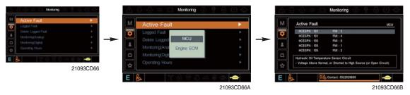
$\cdot\,$  The active faults of the MCU or engine ECM can be checked by this menu.
